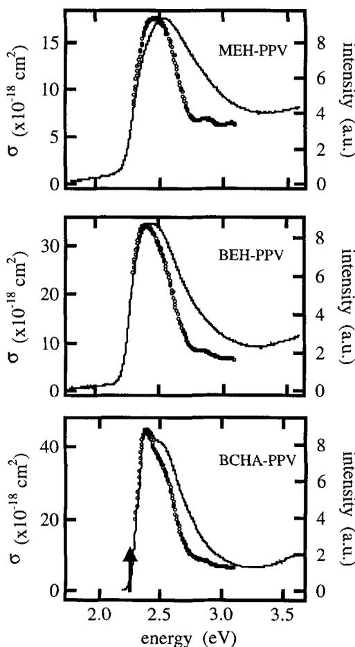
Figure 2: PPV derivative absorption (—) and excitation (o) profiles
