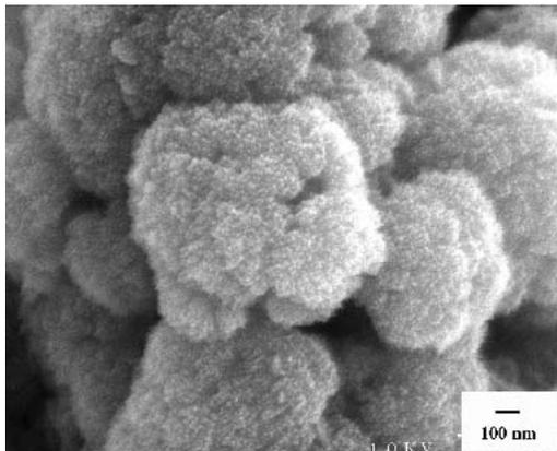
FIG. 5. Cauliflower-shaped, spherical agglomerates of rutile powders are present during the early synthesis stage.
