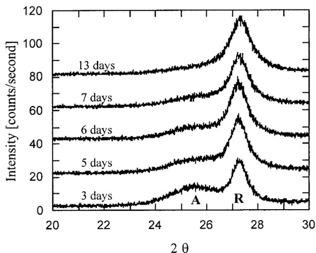
FIG. 2. XRD scans for a sample reaggregated at 65 °C.
