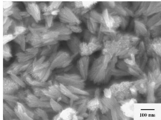
FIG. 7. Small broomlike particles are visible after about 90 days of hydrothermal treatment at 45 °C.
