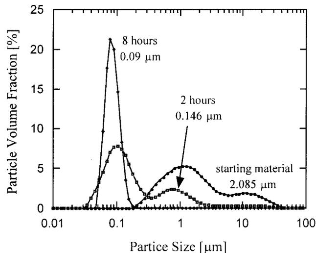
FIG. 10. Particle size distribution for powders hydrothermally treated at 150 °C for 2 to 8 h.
