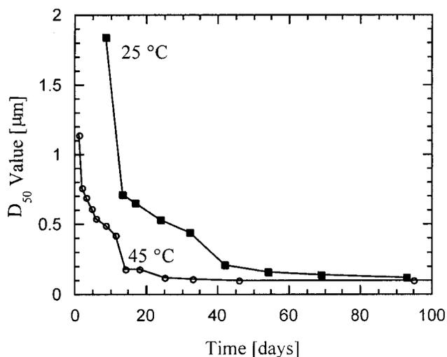
FIG. 9.  $D_{50}$  value as a function of reaction period for samples treated at 25 and 45 °C.
