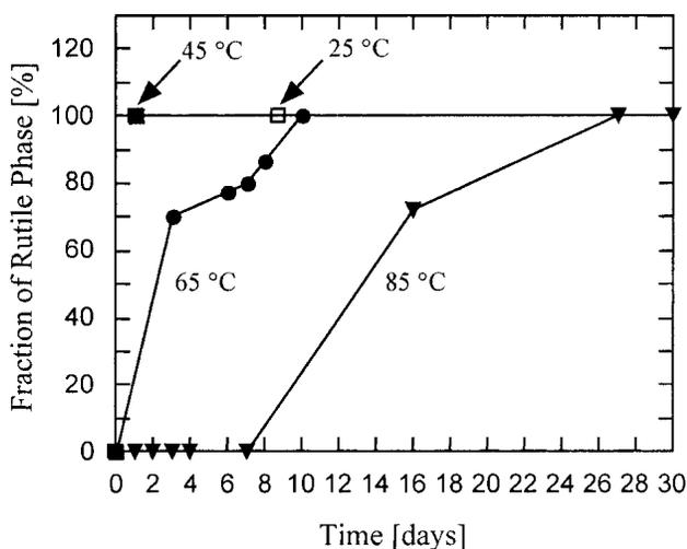
FIG. 1. Phase composition of titania powder samples synthesized at 25, 45, 65, and 85 °C during periods of up to 30 days.
