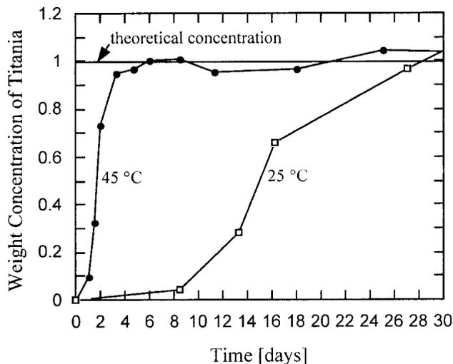
FIG. 3. Weight concentration of rutile powders synthesized at 25 and 45 °C as a function of synthesis period.
