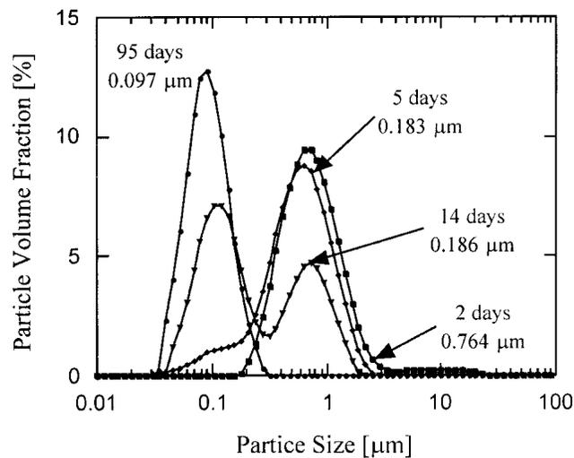
FIG. 4. Particle-size distribution for rutile titania powders re-aggregated at 45 °C.
