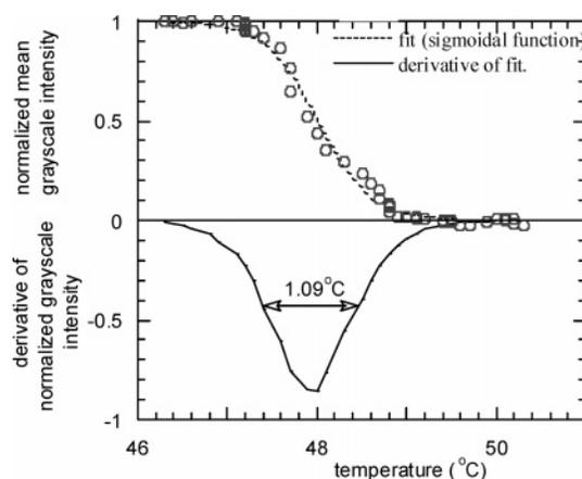
**Figure 10.** Normalized mean gray intensity versus temperature for the dissociation of a two-component aggregate at 70 mM  $\text{Na}^+$  concentration. The dotted line is a fit of the data with a sigmoidal function. The full line is the derivative of this fit, showing the fwhm.
