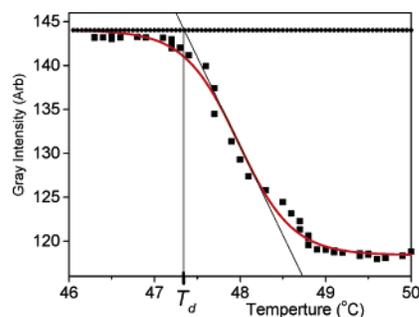
**Figure 4.** Analysis method for determining aggregate dissociation temperature, which is found to be 47.3 °C for the data presented in Figure 3. The red line is a fit with a sigmoidal function. The dissociation temperature,  $T_d$ , is the temperature of the point of intersection of the upper horizontal line determined using the sigmoidal fit and the line fit to the curve at the point of inflection of the sigmoid. Not all data points have been shown in the figure for clarity.
