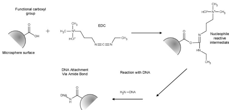
**Figure 2.** Mechanism for attaching amino-modified oligonucleotide to carboxyl-functionalized microspheres.
