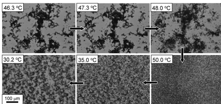
**Figure 3.** Dissociation and reaggregation of a two-component aggregate at 70 mM [Na<sup>+</sup>]. Top Left: the beginning aggregate below dissociation temperature. Following the arrows, the sample is heated above the dissociation temperature ( $T_d = 47.3$  °C) and then allowed to cool. See Figures 4 and 8 for the mean gray intensity measurements and temperatures.
