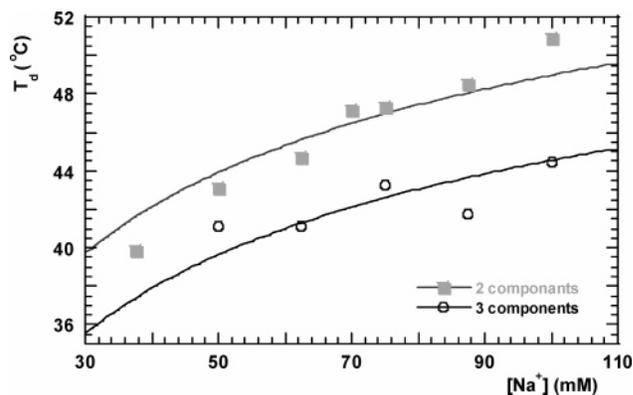
**Figure 7.** Dissociation temperature versus ionic strength for both three- and two-component aggregates. The full lines are a fit of the data points with eq 1, with one free parameter, the dissociation temperature at 50 mM  $\text{Na}^+$ .
