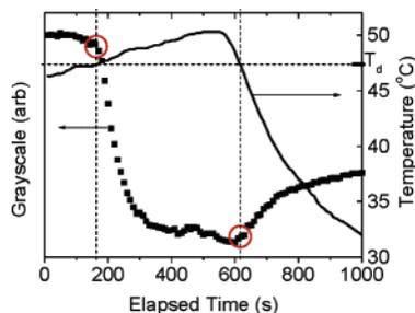
**Figure 8.** Mean gray intensity (squares) and temperature (line) for the dissociation and reaggregation for the data presented in Figure 3. Circled data points correspond to 47.3 °C, the aggregate dissociation temperature.
