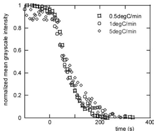
**Figure 9.** Normalized mean gray intensity versus time for the dissociation of a two-component aggregate at 70 or 75 mM  $\text{Na}^+$  concentration. The time  $t = 0$  has been set for  $T = T_d$ . The rate of microspheres dispersion does not increase when the ramping rate of temperature is increased from 0.5 up to 5 °C/min.
