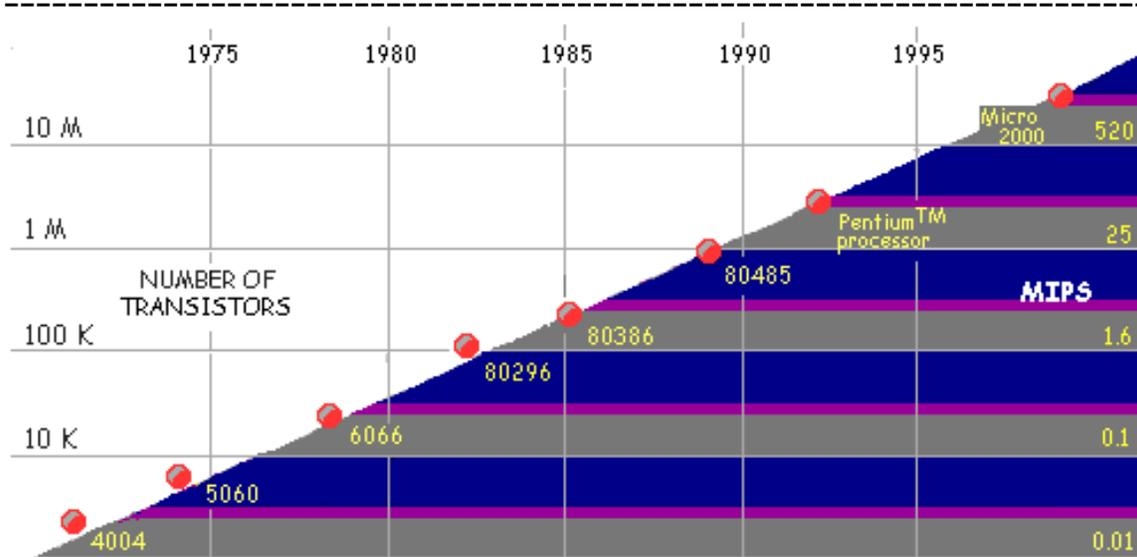
**Figure 3. Moore's Law.** In 1965, Intel co-founder Gordon Moore predicted transistor density on microprocessors would double every two years. This prediction, so far, has proven amazingly accurate. If it continues, Intel processors should contain 50 to 100 million transistors by the turn of the century and execute 2 billion instructions per second (2000 MIPS).
