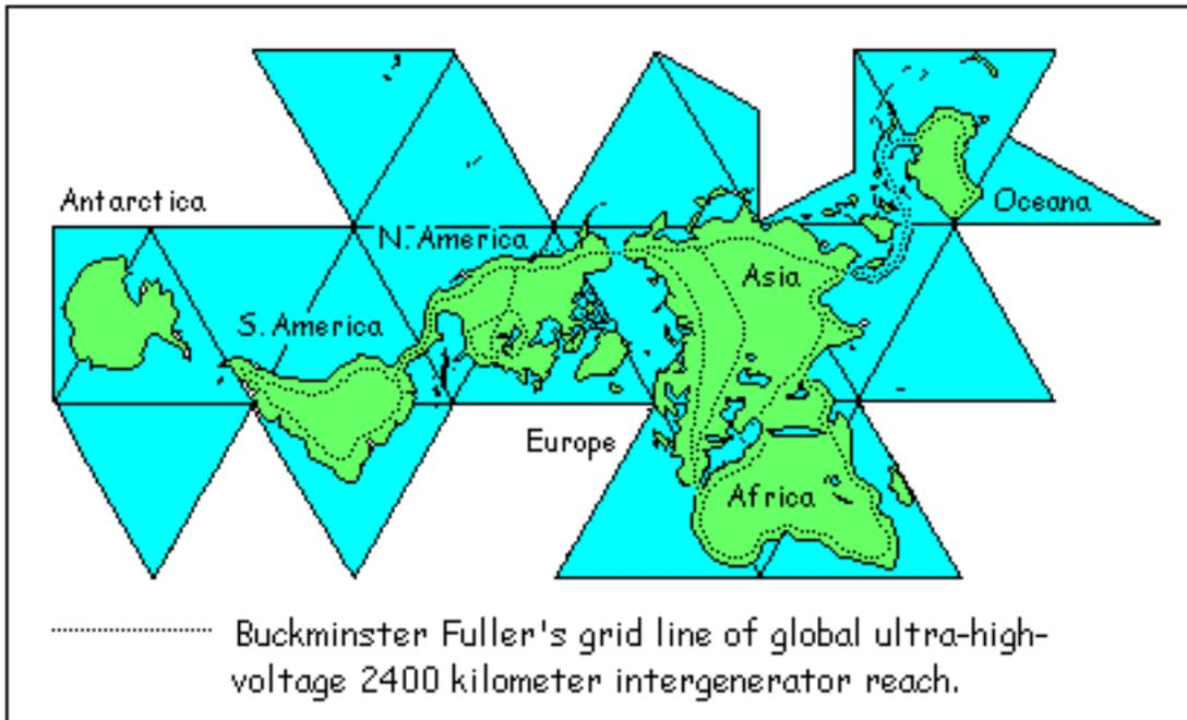
**Figure 4. Prototype global electric power grid based on ultra-high -voltage grid proposed by Buckminster Fuller before the discovery of high-temperature superconductivity. This icosohedral map projection pioneered by Fuller shows the size of the world's land masses and oceans more realistically than Mercator projections, and emphasizes near-contact points where undersea connections to superconducting overland transmission lines could be made (Fuller, 1981).**
